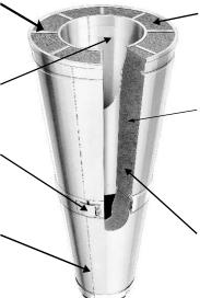
**Insulation-to-Insulation Contact** Creates a continuous column of protection which eliminates cold air infiltration at every chimney joint. This feature significantly reduces the formation of creosote and therefore the potential for chimney fires.
